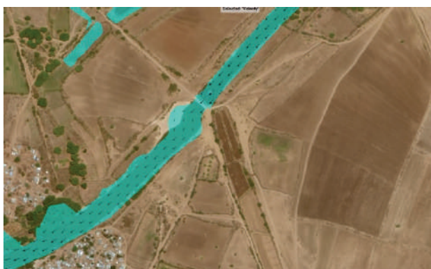
Subset model near Sabuun Barrage to review the flow distribution around the structure
